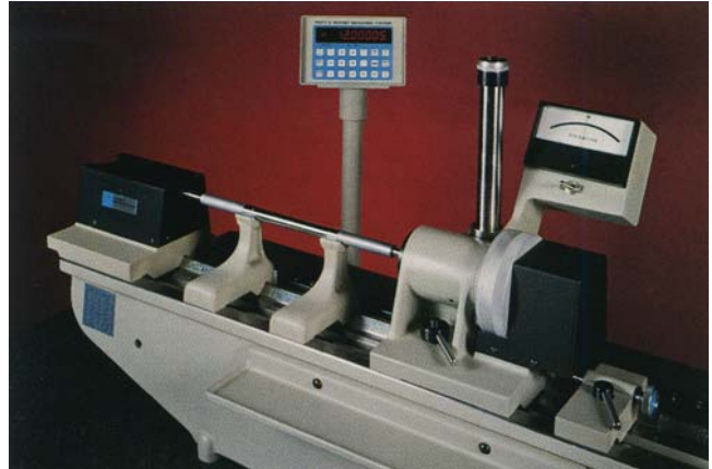
Verifying a Precision end measure length
